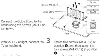
Stand using five screws (M4 X L12) as shown.
